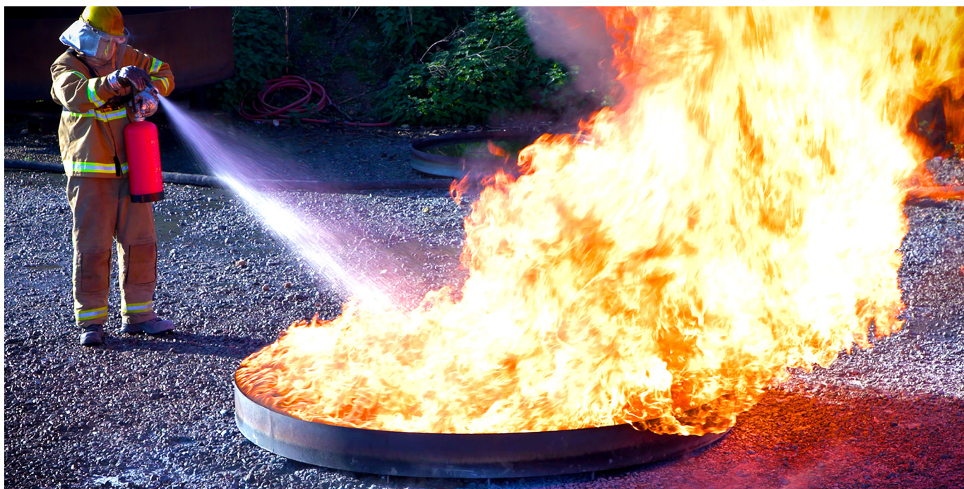
PFAS Free Foam in action on EN3 113B Tray Fire
