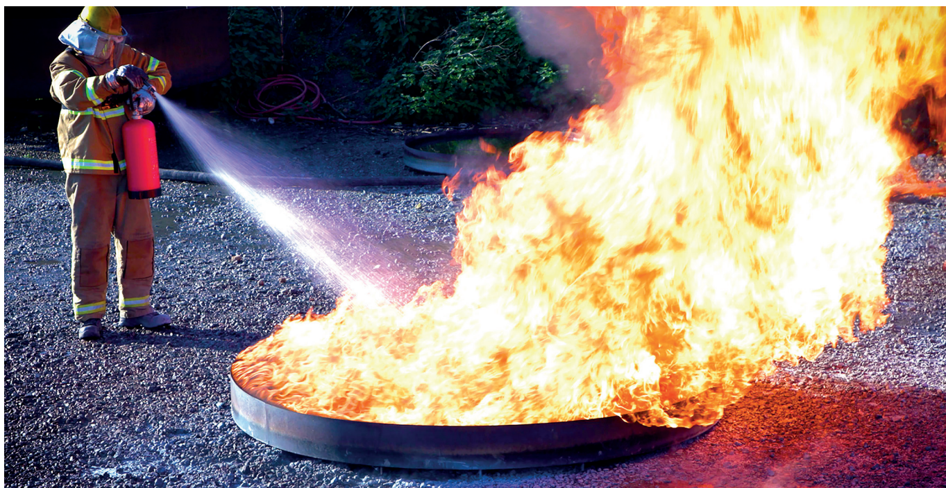
PFAS Free Foam in action on EN3 113B Tray Fire
